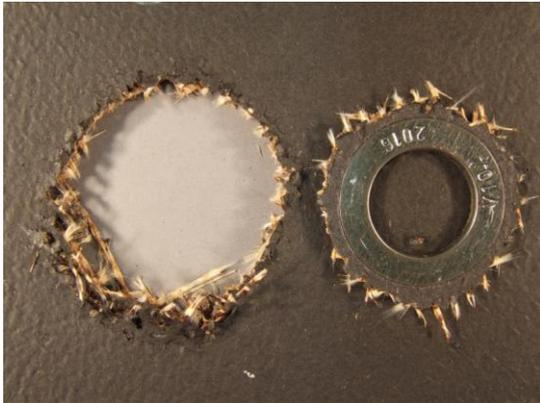
**Type b)** Breakage at bore area
